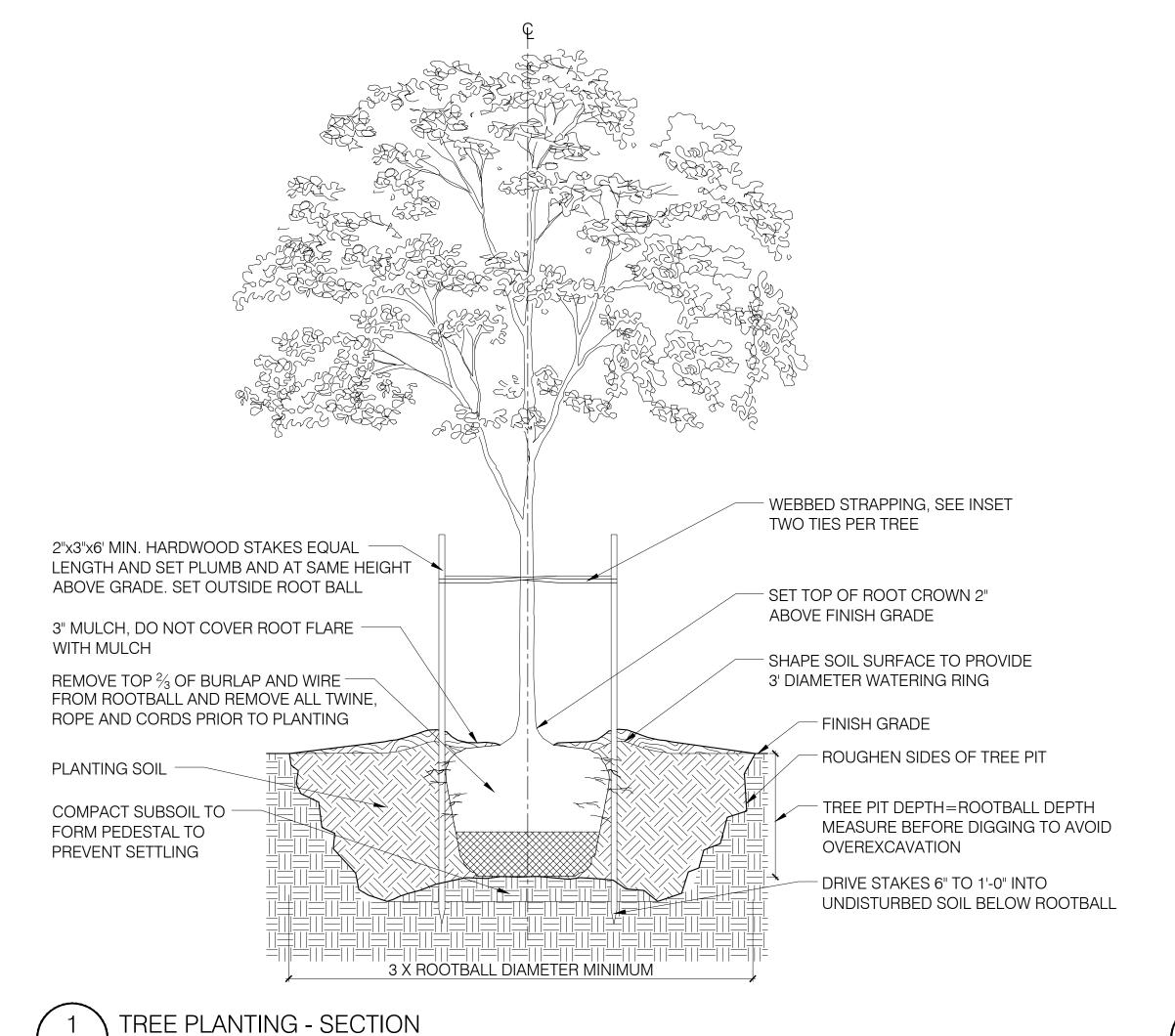
SET TOP OF ROOT CROWN 2" ABOVE ADJACENT FINISH GRADE — 3" MULCH - SHAPE SOIL SURFACE TO PROVIDE 3' DIAMETER WATERING RING — FINISH GRADE ROUGHEN SIDES OF HOLE - AMENDED SOIL TREE PIT DEPTH=ROOTBALL DEPTH MEASURE BEFORE DIGGING TO AVOID OVEREXCAVATION 2 X ROOTBALL PREPARE SUBSOIL TO FORM DIAMETER MINIMUM PEDESTAL TO PREVENT SETTLING NOTES:
