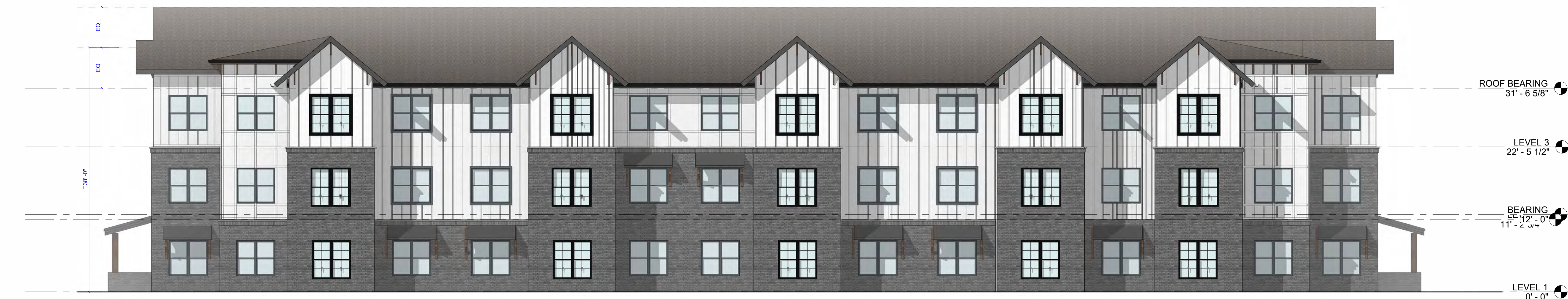
1 BUILDING A FRONT ELEVATION 1/8" = 1'-0"
