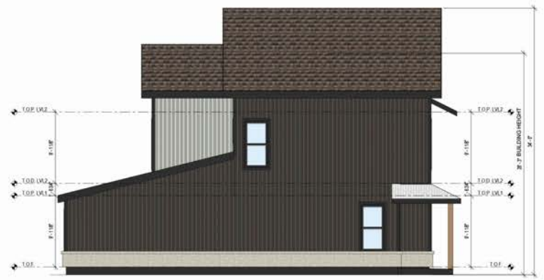
3 BUILDING F - LEFT SIDE ELEVATION 3/16" = 1'-0"
