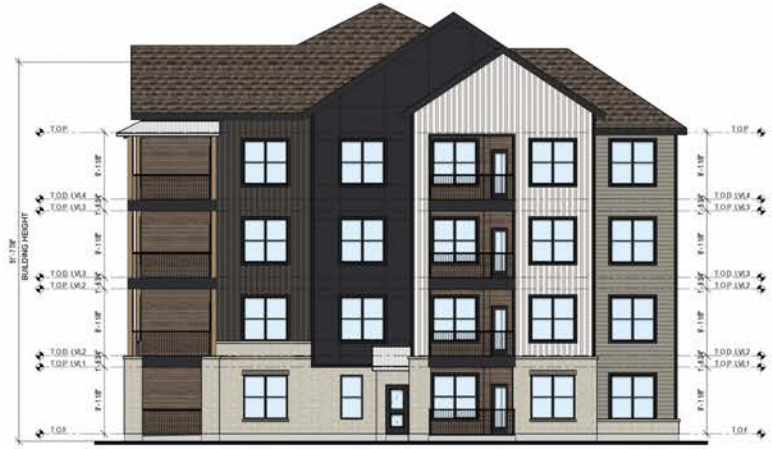
3 BUILDING B - RIGHT SIDE ELEVATION 1/8" = 1'-0"
