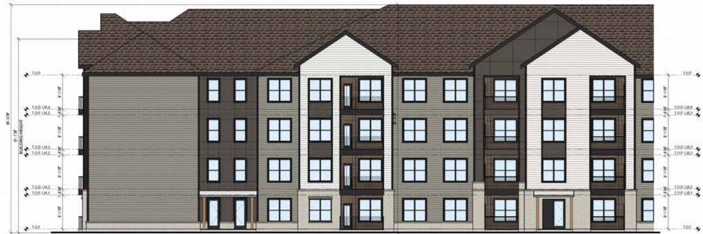
2a BUILDING B - REAR ELEVATION - SECTION A 1/8" = 1'-0"
