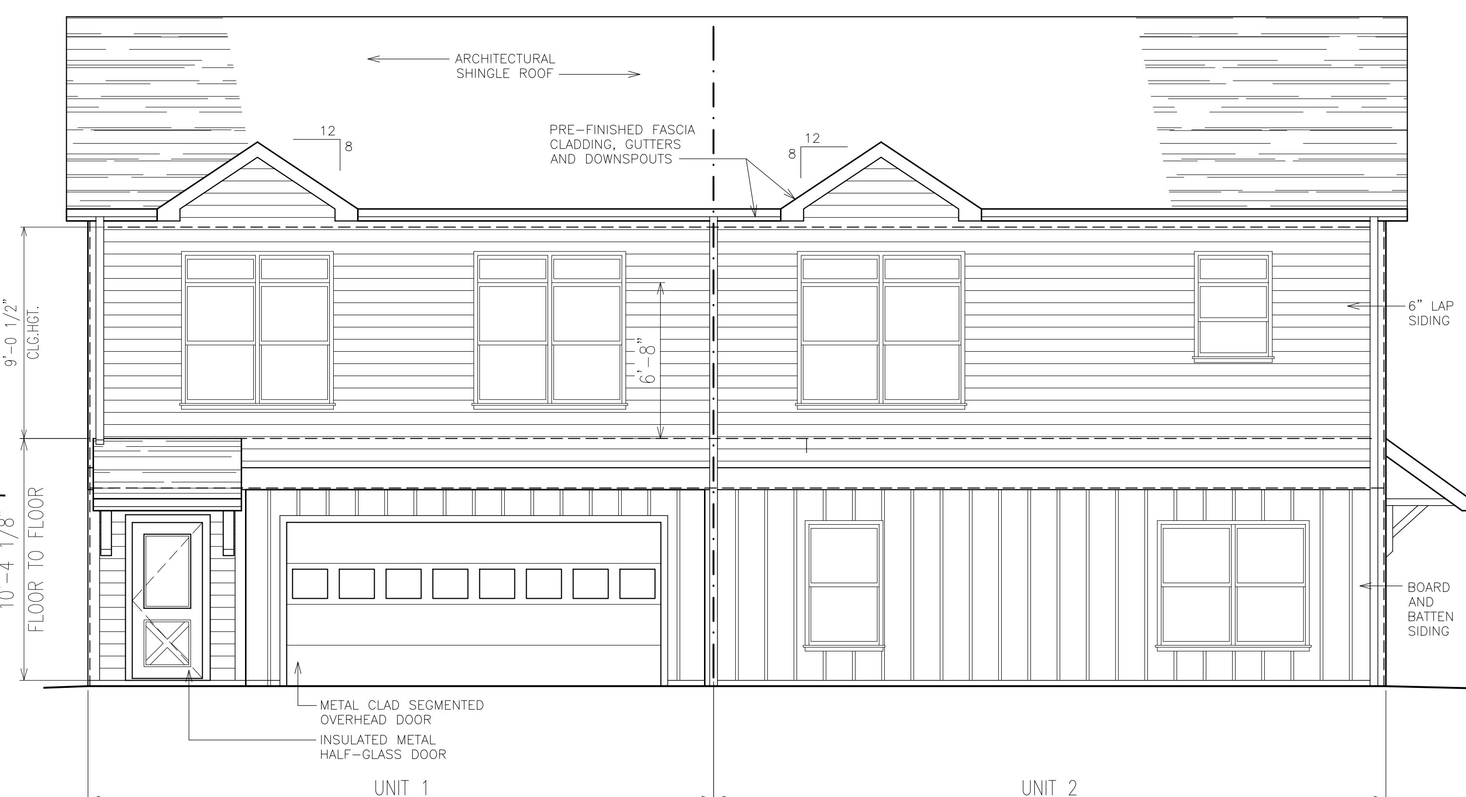
A1 FRONT (SOUTH) ELEVATION 1/4" = 1'-0"
