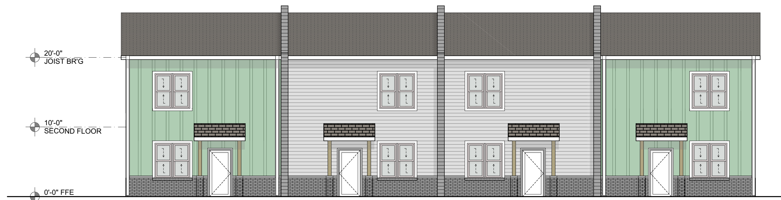
3 TOWNHOME FRONT ELEVATION A1.1 SCALE: 1/8" = 1'-0"
